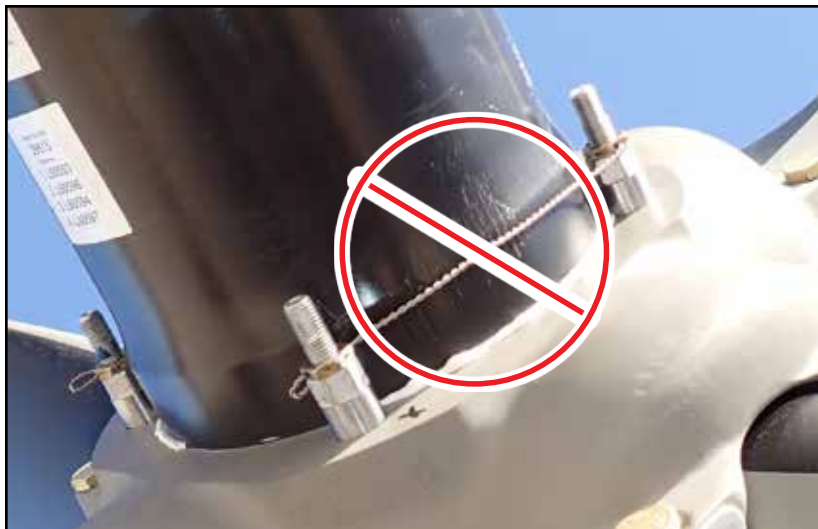
Do NOT Safety Wire the Cylinder-end Beta Rod Nuts Figure 3-3.1
