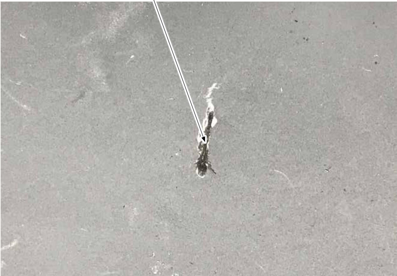
Gouge/Loss of Composite Material
