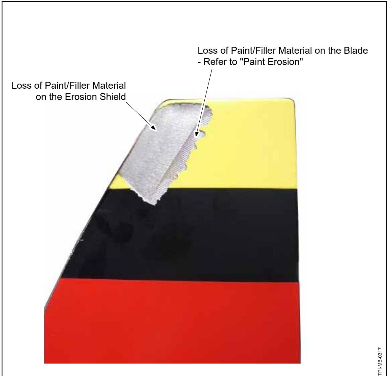
Erosion Shield: Loss of Paint/Filler Material Figure 2-5
