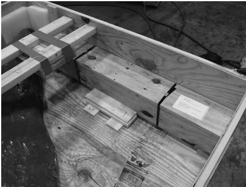
Securing the Box Containing the Beta Valve Assembly Figure 3-6
