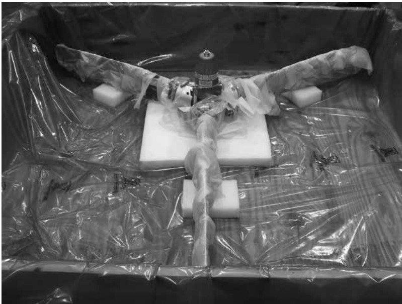
Putting the Propeller on the Foam Blocks Figure 3-2
