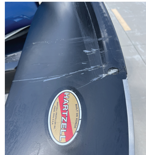
Carbon fiber blade with repairable bird strike damage
