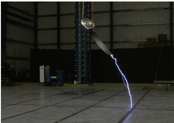
High-voltage lightning strike testing
