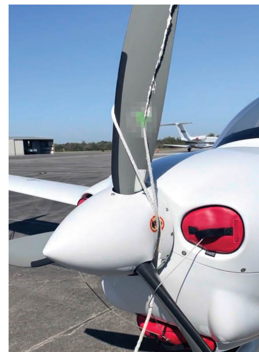
Wood composite irreparable tie down rope damage
