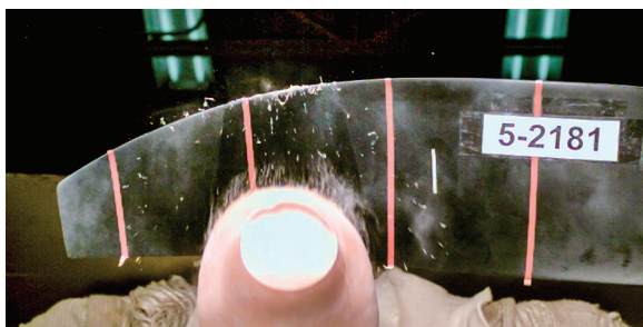
Bird strike testing with 4-lbs weight
