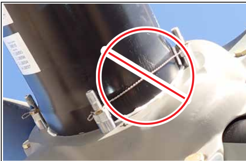
Do NOT Safety Wire the Cylinder-end Beta Rod Nuts Figure 3-3
