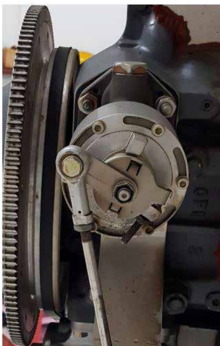
Example of an Installed Governor Figure 3-7
